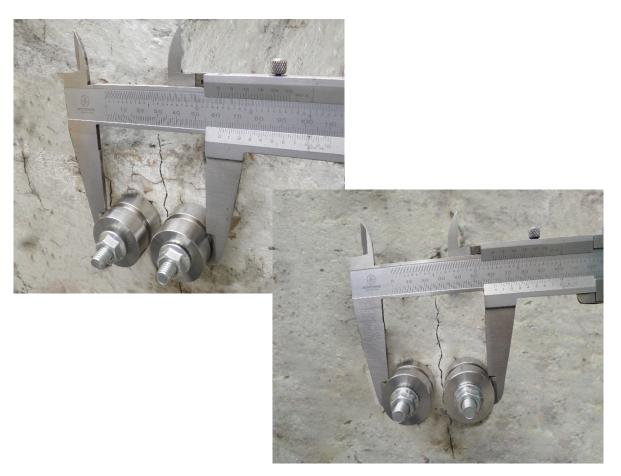
Figure 4: Taking readings of the datum/mounting blocks with Vernier Caliper
